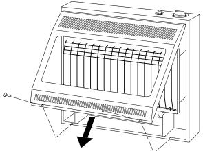
Figure 6 - Removing Front Panel Of Heater
